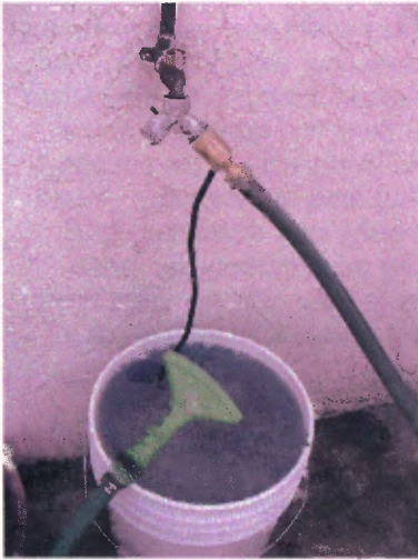
Figure 1. Syphonject hose attachment with 5-gallons of water-soluble concentrate and recommended sprinker wand. This setup provides 85 gallons of water with consistent fertilizer dose
